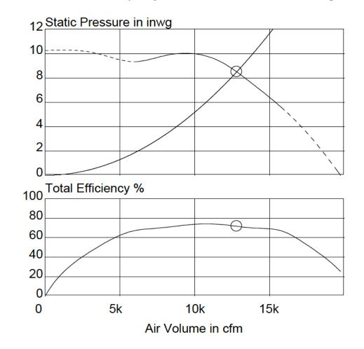
Blower Data: 60HZ curve below. Unit may be operated above 60HZ in VFD mode with higher airflow
